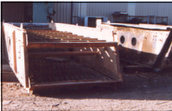
Vibration Screen Deck fatigue nearly eliminated.
